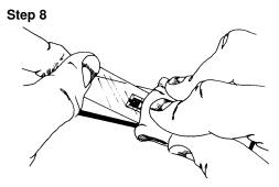
Lift the tucked-over end of tape and bridge it over the adhesive at approximately a 30-degree angle. With a piece of gauze, slowly make a single wiping stroke over the gage/tape assembly, bringing the gage back down over the alignment marks on the specimen. Use a firm pressure with your fingers when wiping over the gage, since the adhesive is quite viscous. A very thin layer of adhesive is desired for optimum bond performance.
