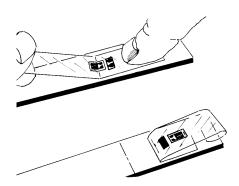
Lift the gage end of the tape assembly as shown here at a shallow angle to the specimen surface (about 45 degrees) until the gage and terminal are free of the specimen surface.
